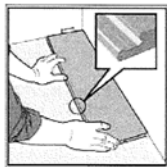
Fig 1. First Row Leave a 10mm expansion gap and begin in one corner working from left to right with the tongue sides of the board towards the wall.
