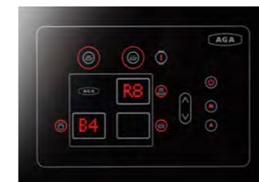
Capacitance touch-screen control
