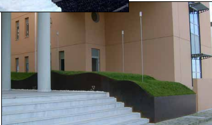
Atlantis Flo-Void® modules used as lightweight structural void fill into landscape planter boxes.
