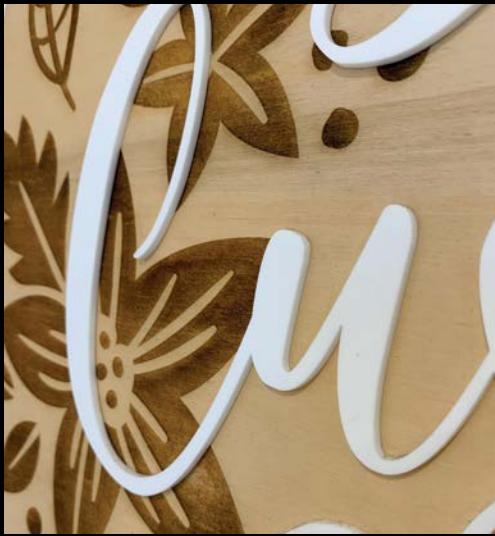
Left: Detail of laser engraving and cutting by Bec's Custom Cuts
