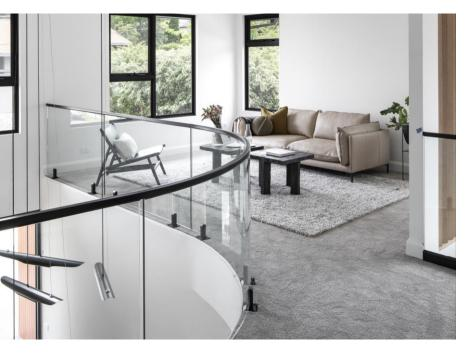
The spigot is our most popular style for frameless balustrades because it is versatile and can be applied to so many different surfaces, whilst providing a minimalistic design. Both durable and desirable with two spigots per glass panel. Often finished with a top rail if required (pictured).
