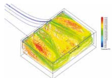
**Figure 4** Temperature contoured flow trajectories
