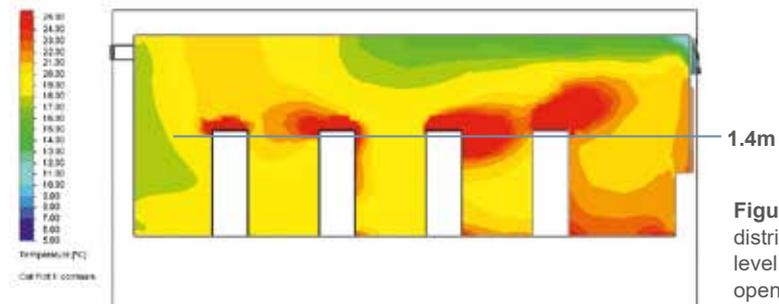
**Figure 2** Temperature distribution for high level top hung outward opening windows
