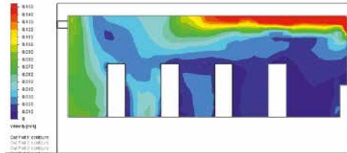
**Figure 5** Air velocity distribution for high level top hung outward opening windows
