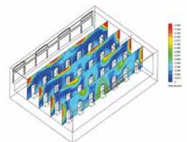
**Figure 6** Air velocity distribution around the occupants
