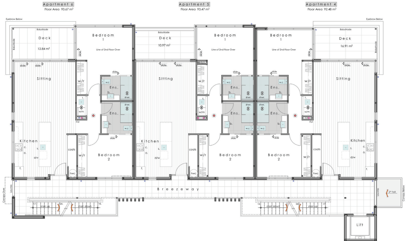
First Floor Plan Scale 1:100 Total First Floor Area 279.63 m 2 Total Balcony Area 40.72 m 2
