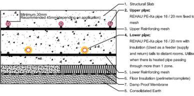
**Typical Floor Structure: In-Slab**
