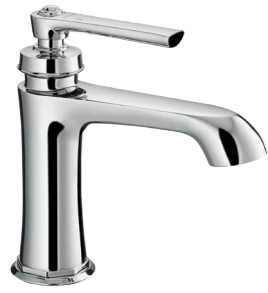
FWL9809CP Standard basin mixer, chrome 100mm aerator height x 130mm reach WELS 5 star 5L/min
