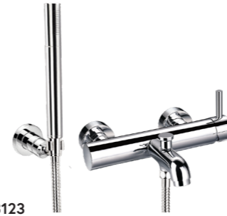
FWE8123 Wall mounted bath mixer and remote mount 185mm reach and adjustable 130mm - 170mm wide 15mm male wall connections handshower set
