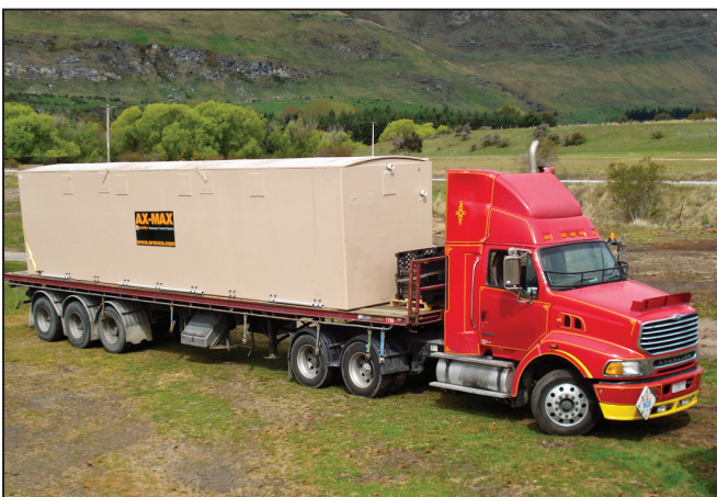
Completely pre-packaged and built inside a durable, insulated, fiberglass tank, an AX-Max™ unit is easy to ship—either by truck, rail, or cargo container.
