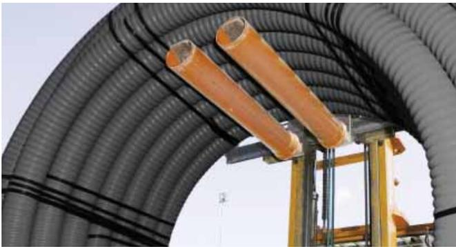
Fig. 41 Lifting with a forklift
