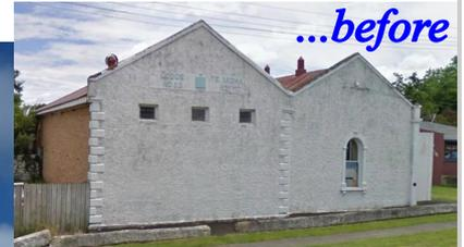
This historical building with majestic mouldings was originally constructed in 1884. Due to 128 years of exposure to the elements, the building was completely dismantled and reconstructed, including using some of the original bricks.
